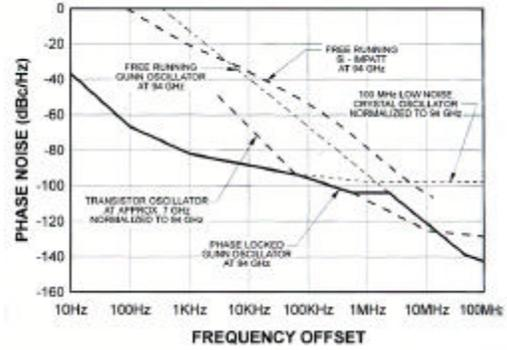
**Figure 3.** Typical Source Noise Characteristics
