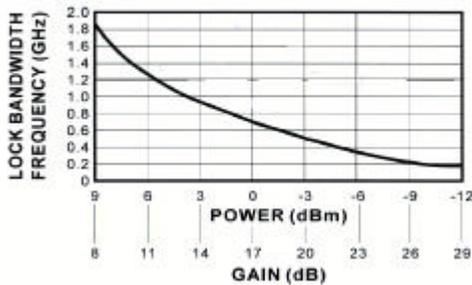
**Figure 2.** Gunn Injection-Locked Oscillator Performance
