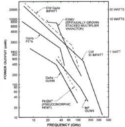
**Figure 1.** Solid-State Source Devices.
