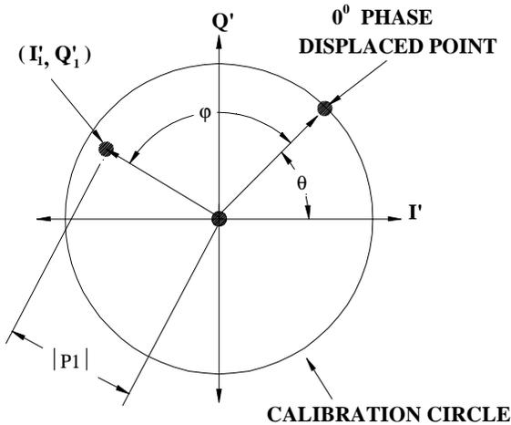
Figure 9: Phase Measurement
