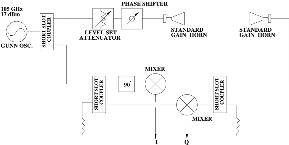
Figure 1: Block Diagram of I/Q Interferometer
