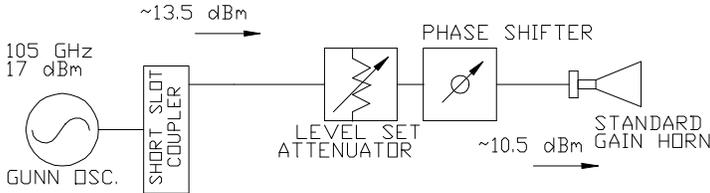
Figure 2: Transmit Hardware
