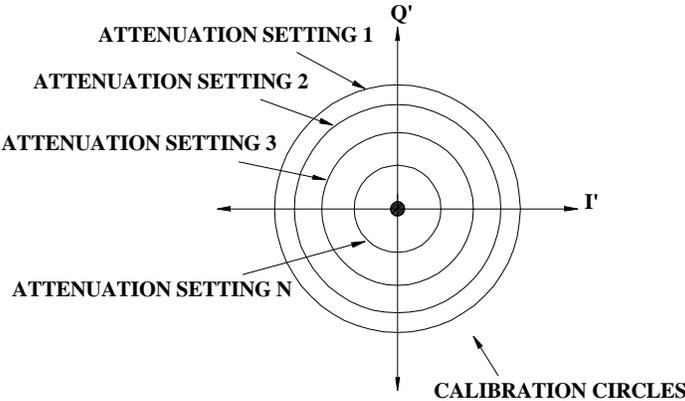
Figure 8: Set of Calibration Circles
