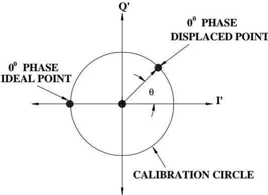
Figure 7: Ideal versus Displaced 0° Phase Point
